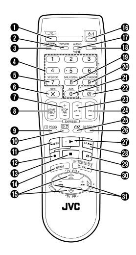
Buttons with a small dot on the left side of the name can also be used to operate your JVC TV while holding down the **TV** button. ( "Operating JVC TVs" in the right column )
